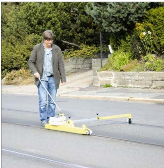
Figure 2. Example of field measurement of rail corrugation.
